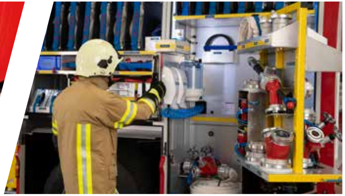
Drehfächer G5 - G6 optional Sliding trap in storage rooms G5 - G6
