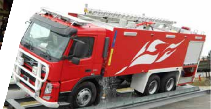
Kipptest Tipping test
