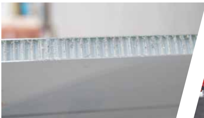
Wabenkernpaneel Honeycombed panels
