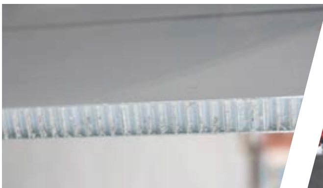
Wabenkernpaneel Honeycombed panels
