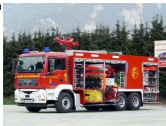
Pumper f. industrial application 4000/2000/1500/240 Plant Fire Brigade Thyssen Krupp/Münchsmünster
