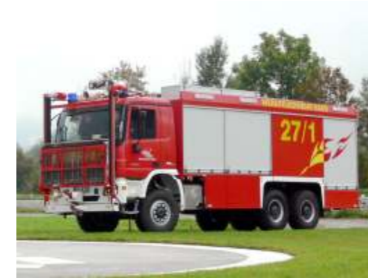
Pumper f. ind. app. 6500 (7500)/1000/500/(240) Plant Fire Brigade EADS Manching
