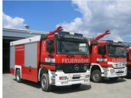
Pumper for industrial application 3000/3000/500 Plant Fire Brigade Refinery OMV Schwechat
