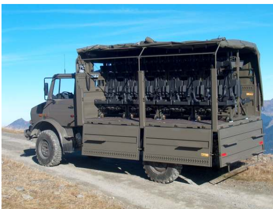
Interchangeable Troop Carrier mounted on: MB UNIMOG U4000
