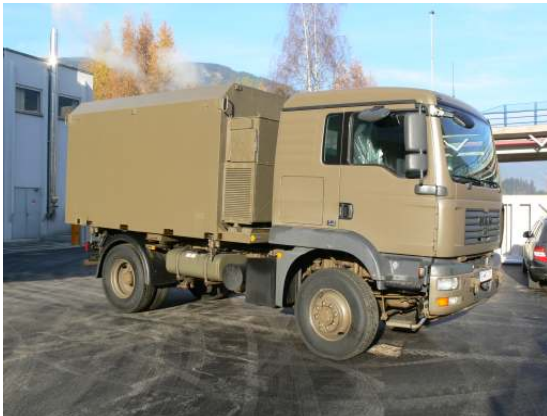
Interchangeable Communication Shelter mounted on: MAN TGM 12.240
