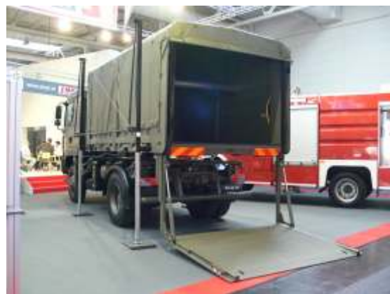
Interchangeable Platform Body with Hydraulic Tailgate mounted on: MAN TGM 12.240
