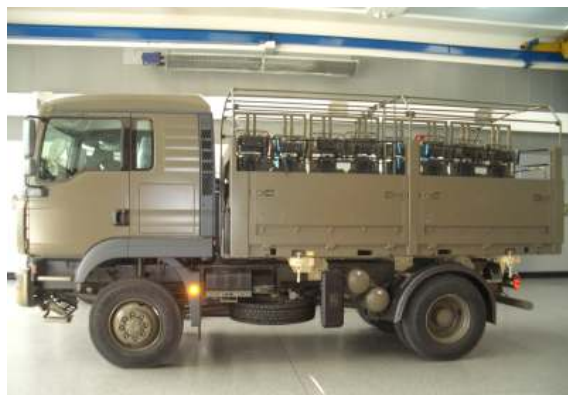
Fig. 3+4: Interchangeable troop carrier mounted on an UNIMOG, MAN & Iveco
