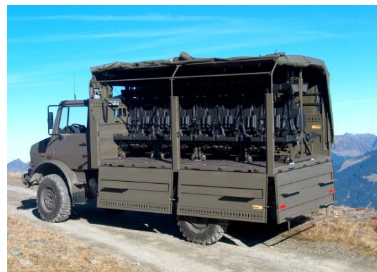
Fig. 3+4: Interchangeable troop carrier mounted on an UNIMOG, MAN & Iveco
