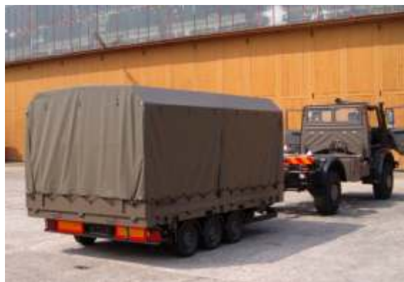
Fig. 5+6: EMPL special low bed trailer for transporting the interchangeable bodies
