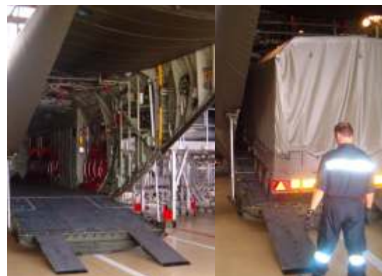
Fig. 5+6: EMPL special low bed trailer for transporting the interchangeable bodies
