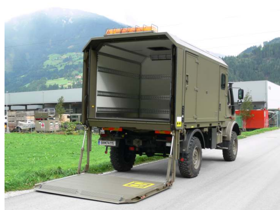
Interchangeable Van Type Body with Hydraulic Tailgate mounted on: MB UNIMOG U4000
