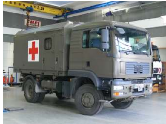
Interchangeable Ambulance mounted on: MAN TGM 12.240
