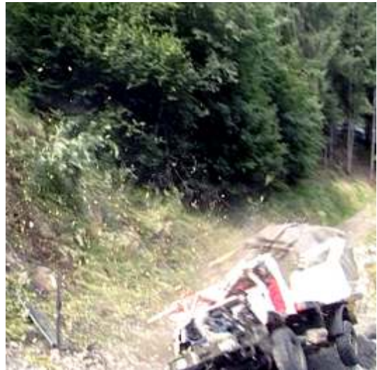
Fig. 29+30: Vehicle after free fall crash (phase 2)
