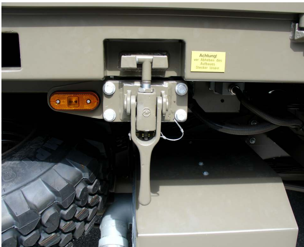
Fig. 3: Locking mechanism for interchangeable body
