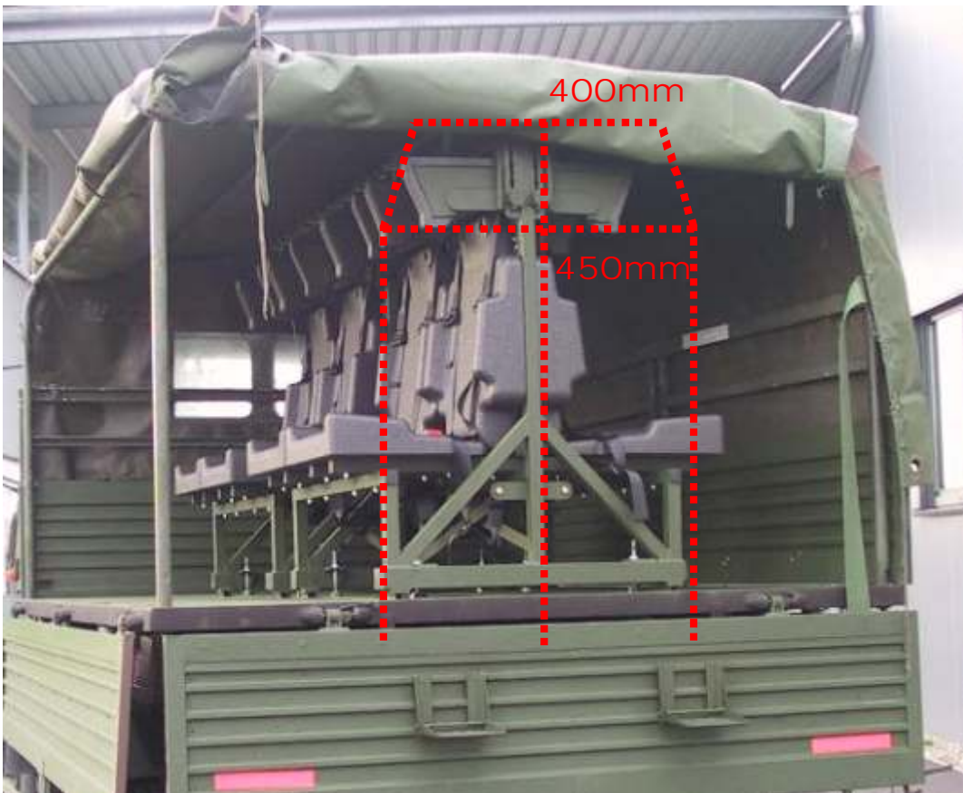
Fig. 5: Defined survival space in the EMPL safety seat module
