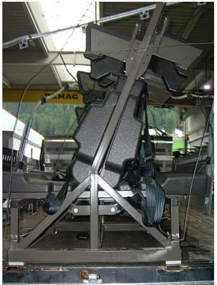
Fig. 34: Safety seat module at the rear
