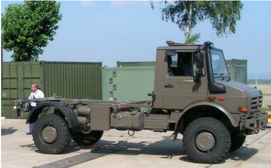
Fig. 2: Vehicle with torsion free subframe
