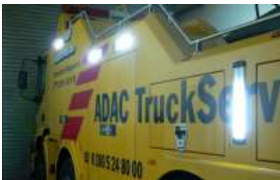
Illumination of operational area on both sides of the compartments
