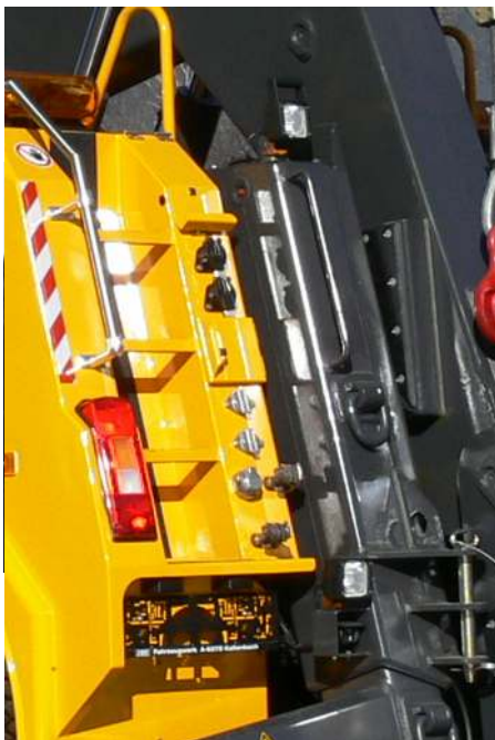
Supply connections for towed vehicles and (semi-) trailers; access ladder with safety railing
