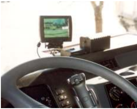
Colour monitor in cab and camera at the rear with working spotlight
