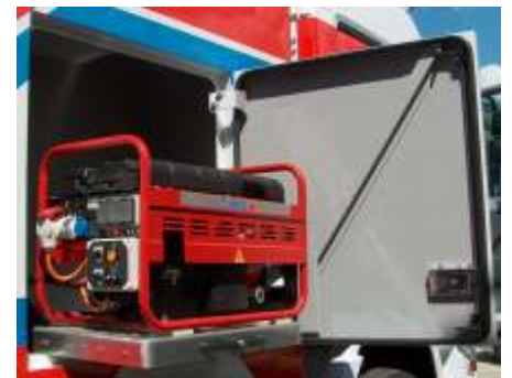
Sliding drawer with generator set for operation of light mast and several recovery accessories
