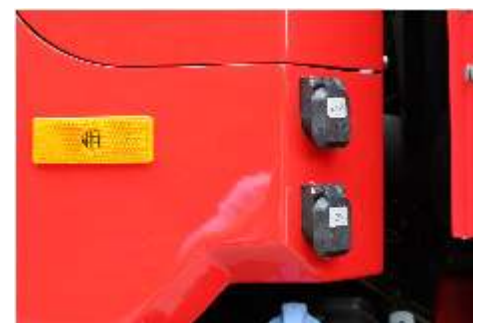
External jump start mechanism either outside of the driver's cab or in the compartment at the rear
