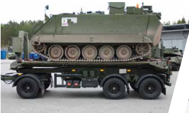
Schlitten-Anhänger Trailer with Sliding Tray
