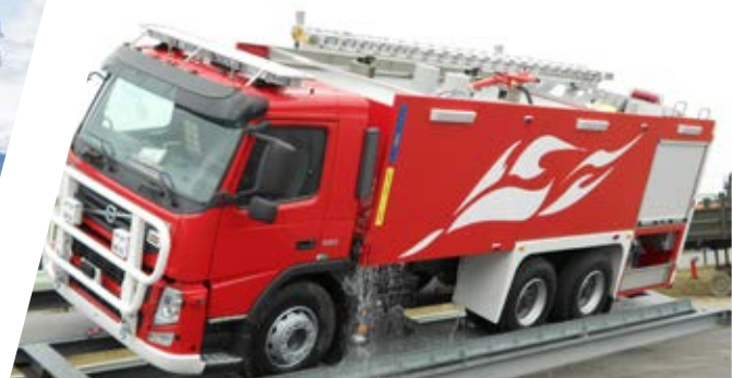
Kipptest Tipping test
