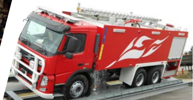
Kipptest Tipping test
