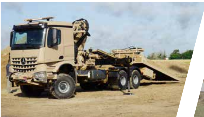
10t Schiebeplateau mit 10t Winde & 3t Hubbrille Sliding Platform, 10to capacity, 10to winch and 3to lifting grid
