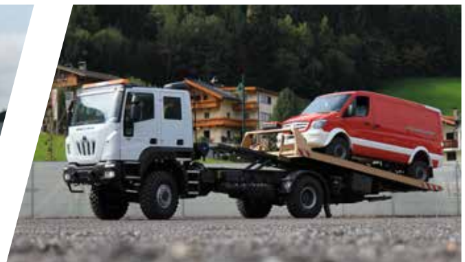
6t Schiebeplateau mit 6,8t Winde & 2t Hubbrille Sliding Platform, 6to capacity with 6.8to winch and 2to lifting grid
