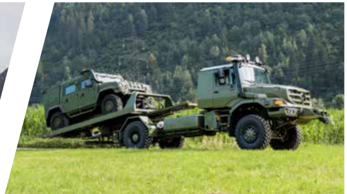
4t Schiebeplateau mit 6t Frontwinde Sliding Platform, 4to capacity with 6to front winch
