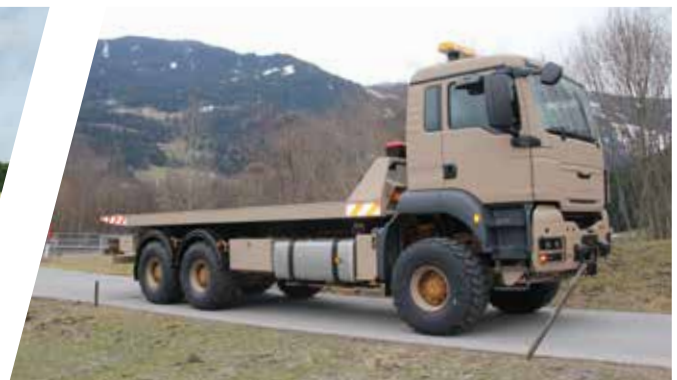
15t Schiebeplateau mit 10t Winde Sliding Platform, 15to capacity with 10to winch
