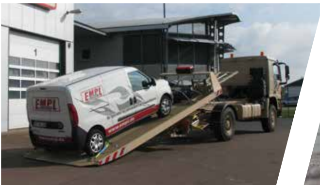
7t Schiebeplateau mit 6t Winde & 3t Hubbrille Sliding Platform, 7to capacity with 6to winch and 3to lifting grid
