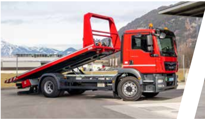
8t Schiebeplateau Sliding Platform, 8to capacity
